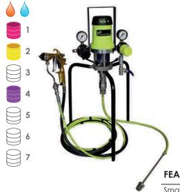
The 10C18 complete Plug & Spray outfit comprises of the pump available in wall-mounted or tripod configuration, the Airmix® Xcite™ 120 bar gun fitted with a 06.094 tip and 7,5m fluid and air hoses in one single package.
